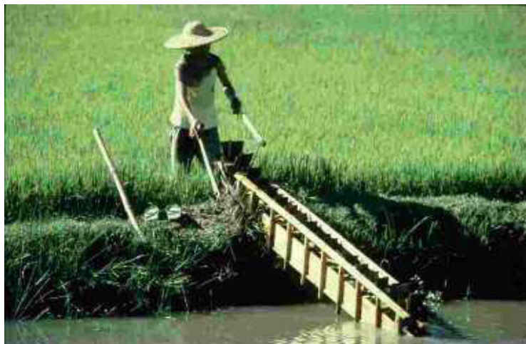
Figure 2: Chinese rice farmer using a hand-operated pump to draw water from a canal
